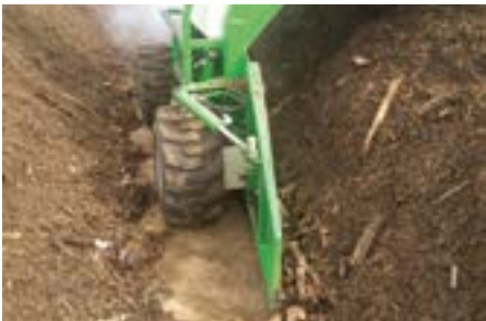
Single swiveling, hydraulic shields ensure clean troughs.
