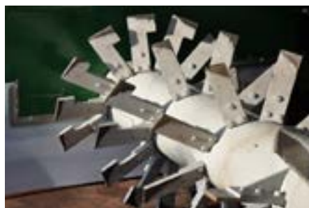
The good turning shaft turns the material from the inside to the outside, so that the microorganisms can be replicated everywhere optimally.
